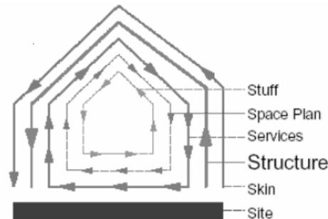
**Figure 3:** The Shearing Layers model (Brand, 1994)
