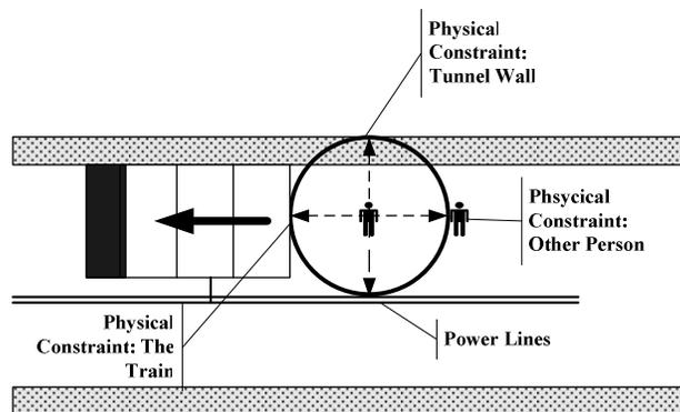
Figure 1: The Field of Comfort for a Passenger Evacuating a Train in a Tunnel
